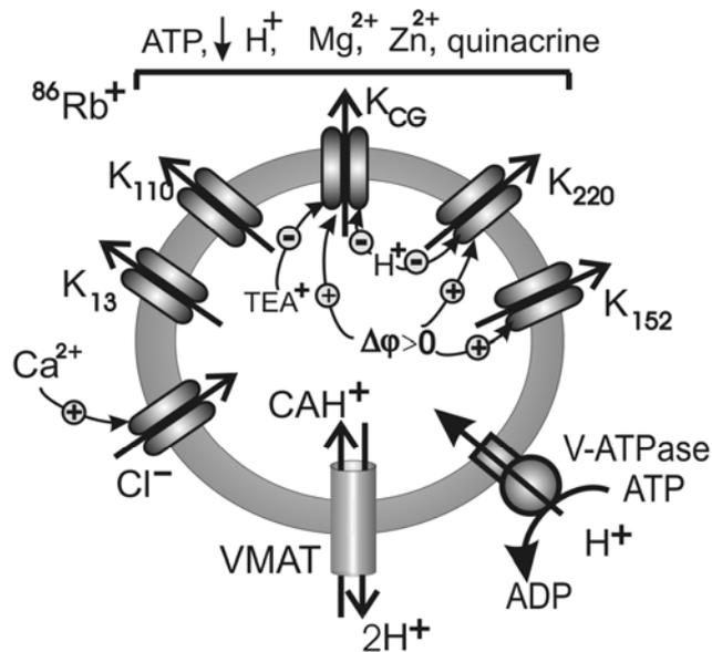
Fig. 6. The channels and transporters of the chromaffin granules. VMAT – catecholamine ( $CAH^+$ ) transporter, V-ATPase – proton pump; there are five potassium channels and one calcium-dependent chloride channel. Adding  $TEA^+$  and lowering pH closes channels, while increasing the potential difference ( $\Delta\phi$ ) opens channels. The  $^{86}Rb^+$  flux experiments and measurements of a single channel in BLM show that potassium conductivity is affected by the same blockers.
