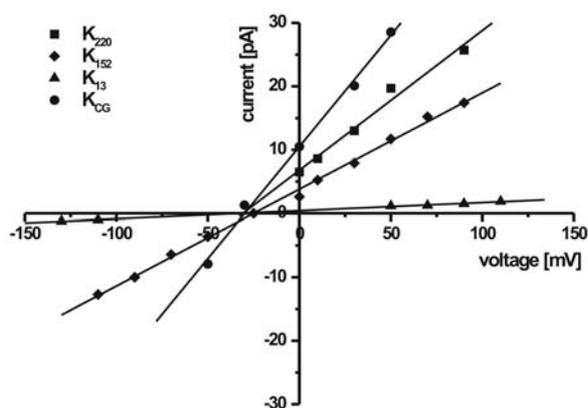
Fig. 3. The current/voltage relationship of the four potassium channels presented in Fig. 2. 450/150 mM KCl, 5 mM HEPES/KOH, pH 7.0 *cis/trans* buffers. The recordings were low-pass filtered at 0.2 kHz. The solid lines are drawn to a linear fit of the data.
