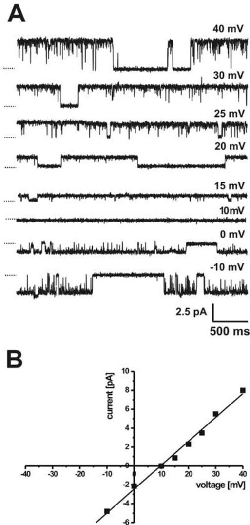
Fig. 5. The anion channel of a chromaffin granule. 500/150 mM KCl, 5 mM Hepes/KOH, pH 7.0 *cis/trans* buffers in the presence of 2 mM  $\text{CaCl}_2$ . A – Single channel recordings. The closed level marked as  $\cdots$ . The recordings were low-pass filtered at 0.2 kHz. B – Current/voltage relationship.
