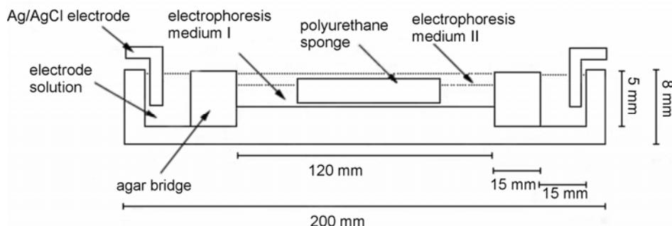
Fig. 1. Diagram of the electrophoresis chamber and the Ag/AgCl electrodes.
