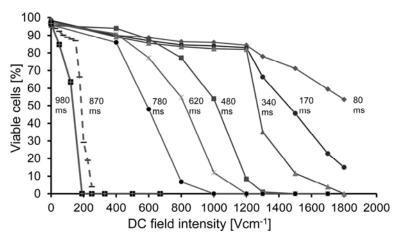
Fig. 6. Viability of AT2 cells exposed to dcEFs of different durations. Each curve corresponds to a different exposure time.
