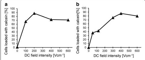
Fig. 6 AT2 prostate cancer cell loading with calcein following a single 80 ms exposure to dcEF. a – Electroporation cuvette system. b – Flow-through electroporation system
