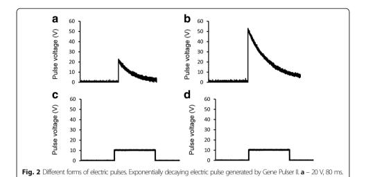
$\mathbf{b}$  – 50 V, 80 ms. Square wave pulse generated by square and double pulse generator.  $\mathbf{c}$  – 10 V, 80 ms.  $\mathbf{d}$  – 20 V, 80 ms
